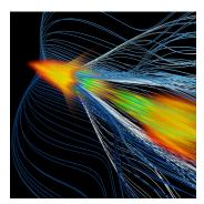
Studies at SLAC's FACET (Facility for Advanced Accelerator Experimental Tests) demonstrated a new, efficient way to accelerate positrons, the antimatter opposites of electrons, by having them "surf" waves of hot, ionized gas in a technique known as plasma wakefield acceleration. The method may help boost the energy and shrink the size of future linear particle colliders that probe nature's fundamental building blocks.
