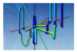
INL's Reactor Excursion and Leak Analysis Program5-3D (RELAP5-3D) is used primarily for analysis of potential accidents and transients in water-cooled nuclear power plants, and for analysis of advanced reactor systems.
